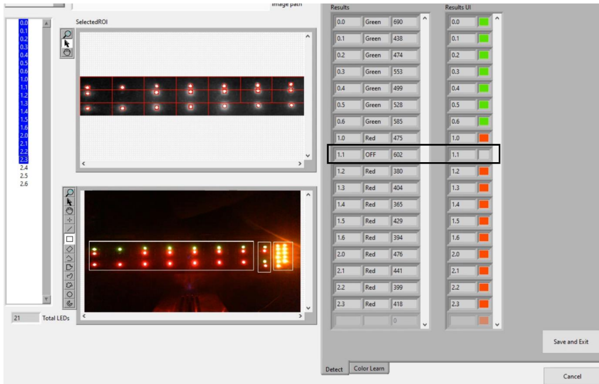
Figure 4: Live view of LEDs operation mode as calculated in software application
